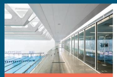
Pools and gyms are notorious for their noise. Mitigating this, ROCKFON Sonar ceiling panels are made from stone wool, an inherently high-performing, sound-absorptive material.
