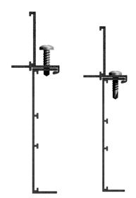
Ensuring that the Transition trim is properly engaged with the Perimeter trim, use #10 Self-drilling screws at 24" on center to fasten the two elements together. Any cuts should be made within 6" of fasteners, or an additional fastener should be added.
