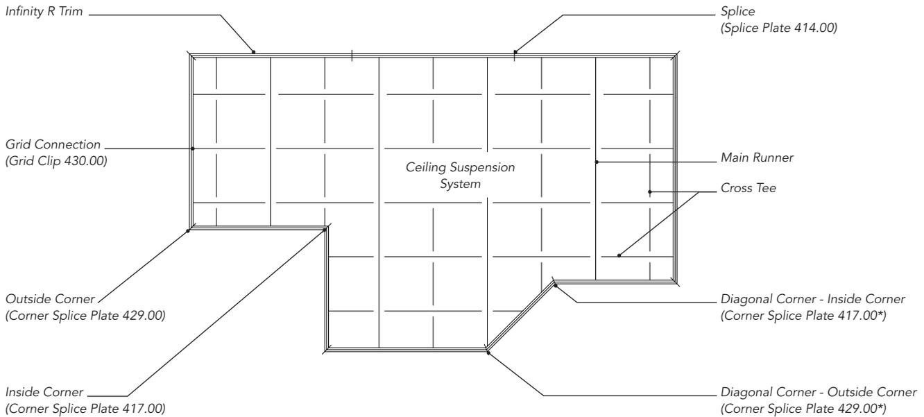
\* Field modify Corner Splice Plate to achieve desired angle greater than or less than 90°.
