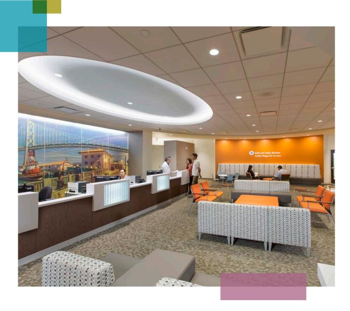
In total, Spacetone Acoustics installed Rockfon Artic®, Alaska® and Hygienic Plus™ acoustic stone wool ceiling panels; Rockfon® Spanair® Torsion Spring concealed metal ceiling panels; Chicago Metallic® Ultraline™ and 1200 Series 15/16-inch ceiling suspension system, and Rockfon® Infinity™ Perimeter Trim.
