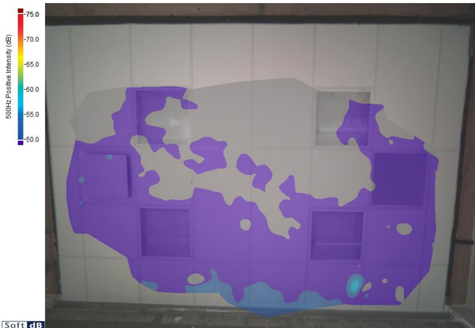
Fig. 5 – A color map showing sound transmission through the ceiling and plenum barrier combination, 500 Hz octave band, stone wool ceiling panels (NRC 0.95, CAC_{panel} 22), double-layer plenum barrier. Using a plenum barrier improved overall performance to CAC_{system} 49.
