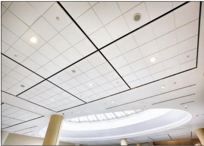
*Suspension systems define the ceiling's visible grid. Coupled with stone wool ceiling panels, the grid can be accentuated with a wide face, minimized with a concealed grid, or recessed for a shadow effect.*
