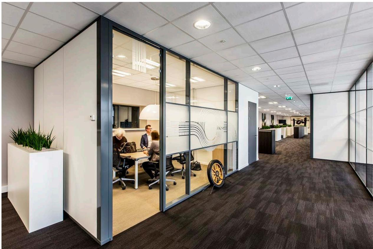
**Figure 1: Architectural and operational trends in commercial interiors of combining demountable partition systems with continuous acoustic ceilings can lead to poor sound isolation because noise travels over the partition through the space above the ceiling.**
