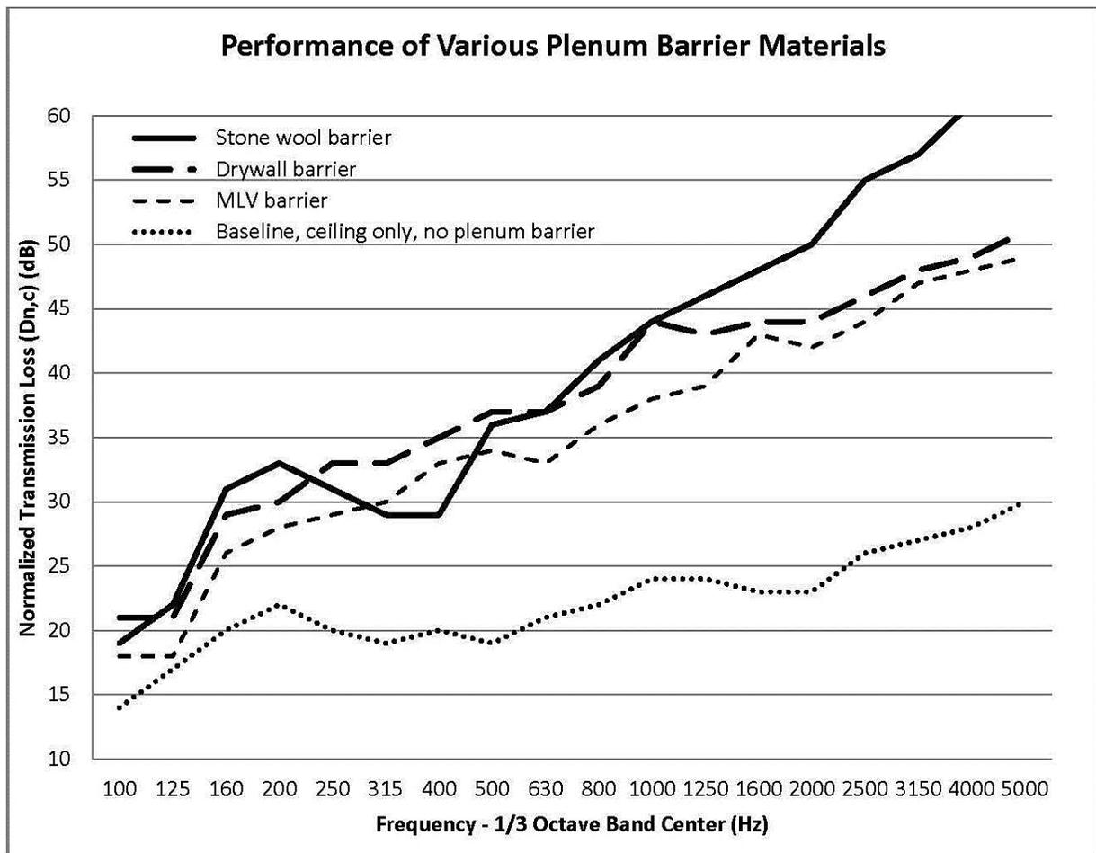
**Figure 5: Laboratory tests show that a single layer of MLV (1/8 inch thick, 1 psf) has lower transmission loss performance than a single layer of GWB (5/8 inch thick, 2.3 psf) and a single layer of stone wool with a foil facing (1.5 inch thick, 1 psf). During these tests, all plenum barriers were penetrated by a supply-air duct, three metal conduits and three PVC pipes that were suspended in the plenum to better represent conditions in actual buildings.**
