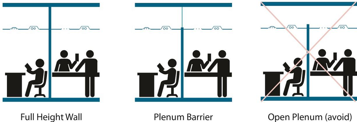
**Figure 3: Three design approaches for sound isolation in commercial interiors: full-height walls that comply with standards and user expectations, but cost more during construction (left); lightweight plenum barriers above partial height partitions, which meet sound isolation requirements at lower cost (center); and partitions that stop at ceiling height leaving an open plenum, which does not work acoustically (right).**
