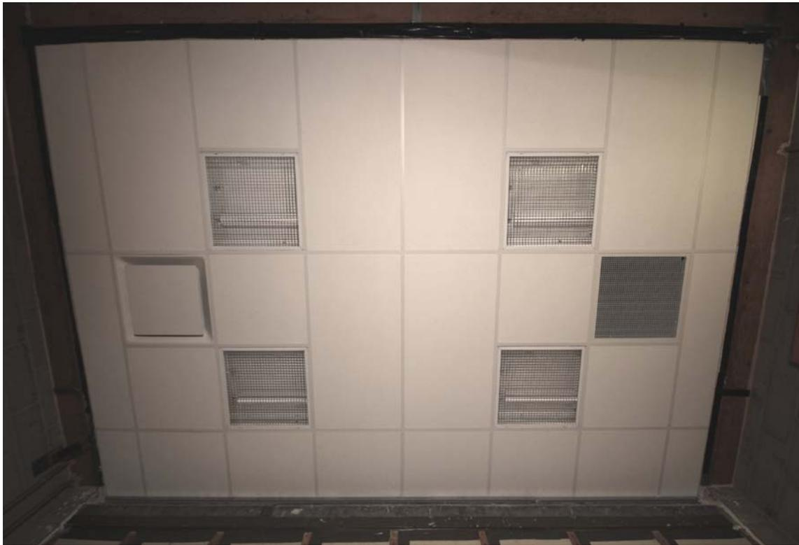
(4a) Image of a ceiling system, representative of a typical office ceiling, installed in a laboratory test chamber; a plaque-style, ducted, supply-air diffuser (left), four recessed light fixtures (center) and an unducted, return-air grille (right). The partition along the bottom of the image is common with an identical room with the same ceiling system and white noise playing at 94 dB through loudspeakers.
