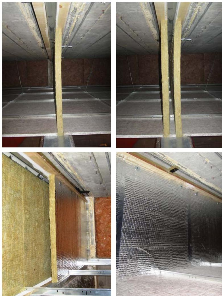
**Figure 10: Lightweight, stone wool, plenum barriers installed above the central demising wall of the laboratory's chamber during testing. Top-left: Single-layer. Top-right: Double-layer with a 1-5/8 inches airspace in between. Bottom-left: Double-layer with seams staggered and small cuts at the bottom so the panels slide down over the grid bulb. Bottom-right: Installation complete with tops screwed, seams taped and ceiling panels installed.**
