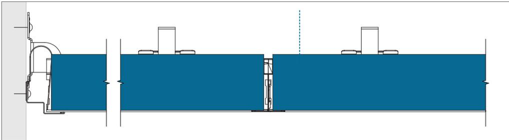
E-edge - Perimeter finish with wall angle trim and wall spring fix.
