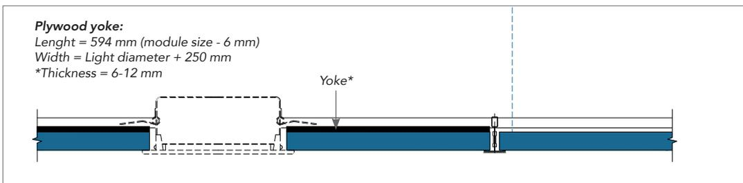
\*The thickness of the plywood or metal yoke needs to be adapted in function of the weight, size and position of your service integration (e.g. downlight or speaker). The Plywood or metal yoke itself may not deflect after installing your service integration.
