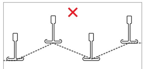
It is also important to check the squareness of the angles between the main runners and cross tees. This can be easily done by comparing the measurements of the two diagonals. See recommended tolerances on the table to the right.
