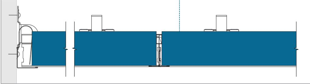
A-edge - Perimeter finish with wall angle trim and wall spring fix.
