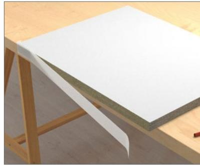
3. Align 5 mm overlap on front and press.
