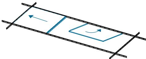
Push the panel so that the open C edge of the panel slides into the 4' cross tee. The 477.00 spline will create the support on the open side. Repeat this process with the opposite side of the 4' x 12' opening.
