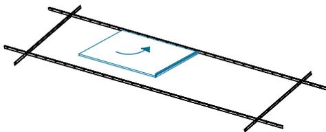
From above the grid, place the SLP panel with one (1) 477.00 spline onto the main runner. Push the panel so that the D2 edge seats into the grid. Allow the panel to come to rest on the opposite D1 edge.
