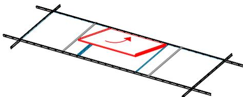
The center panel is the last component to complete a 4' x 12' module. This panel installs the same as the perimeter panels except it remains in the center and both C edges have 477.00 splines installed in them.
