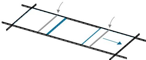
With both edge panels in place, install a 828.00H: 4' spacer bar over the top of both panels just inside of the 477.00 splines.
