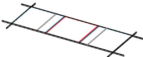
The middle panel is the accessible panel, however if more space is required to access the plenum, reverse the steps above to remove additional panels.
