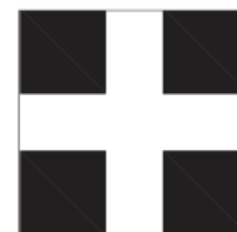
AH 750S1250L 0.75" Square Holes 1.25" Straight Centers 36% Open Area
