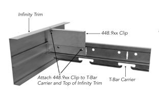
Attaching Infinity to T-Bar Carrier
