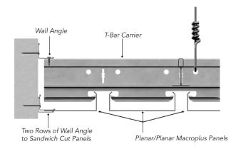
Securing Panels at Perimeter with Wall Angle
