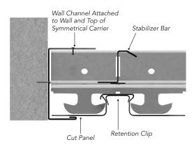
Perimeter Detail Using Channel
