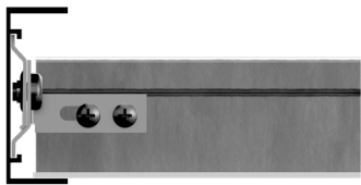
Floating Perimeter with Infinity™ Trim
