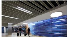
Rockfon® Intaline<sup>™</sup> Round-Base and V-Base vertical baffles can be used to create a field of visual interest or used to define a space. These aluminum baffle ceilings are installed using a standard 15/16" acoustic ceiling grid which installs quickly and integrates with industry standard lighting and air diffusers. Rockfon Intaline baffles are available in a wide variety of finish options including painted colors, wood-look and metal finishes.
