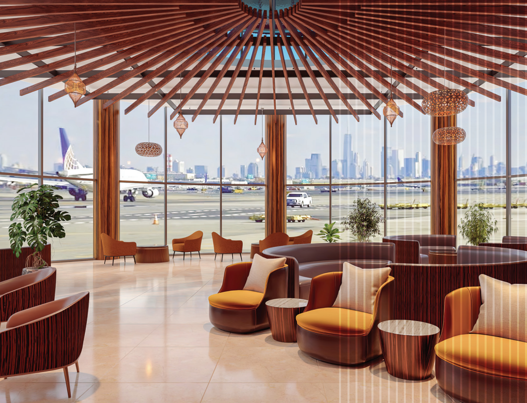
Baffle (W × H): 1" × 6" Baffle Finish: Woodlands™ – #550 Canyon Walnut Installation: Cubegrid® – 08 Black Application: Airport Lounge Lobby – Radial Installation
